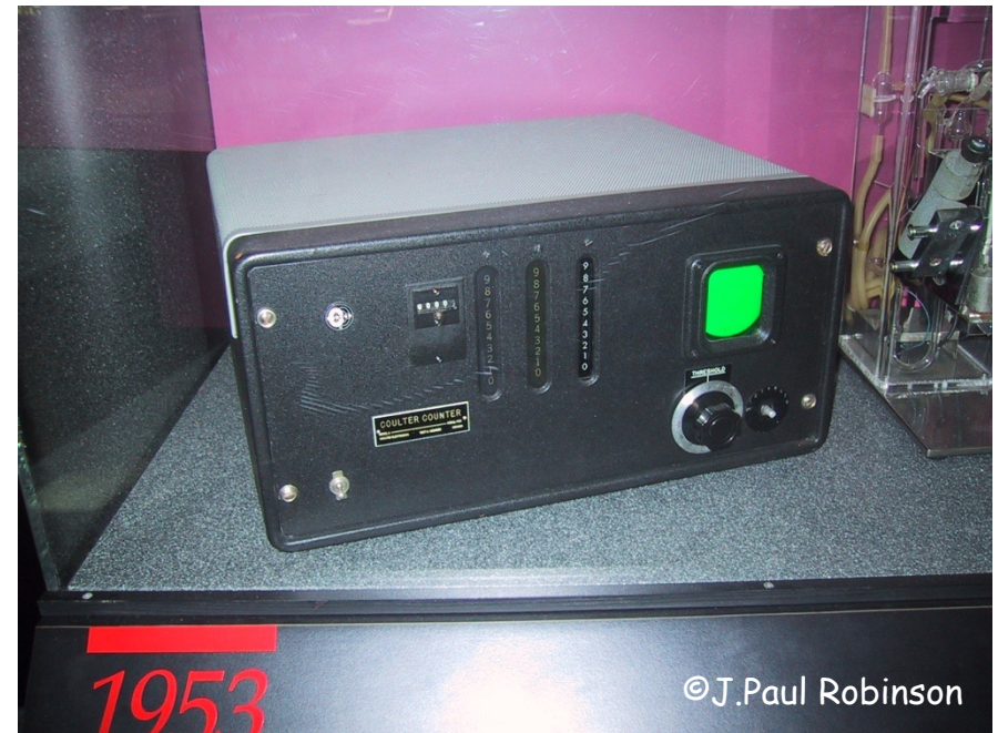
The first commercial version of the Coulter Counter was sold in 1956
