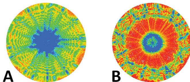
Figure 1. Examples of laser light scatter patterns formed by *E. coli* colonies. A – O157:H7, B – O26:H11. Pseudocolor look-up table added to visualize intensity differences.
