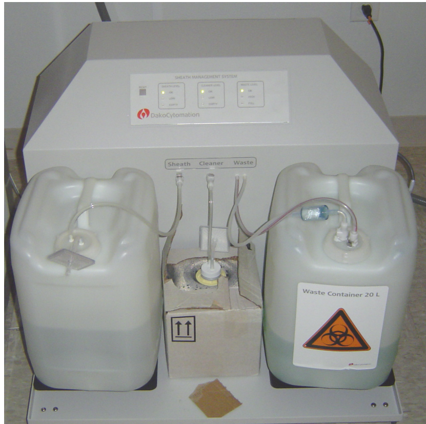
Figure 3.2: SMS front view with reusable sheath and waste tanks and Dako cleanser box.
