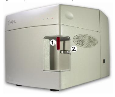
1. Sample Probe with a Sample Tube Loaded
