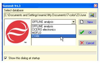
2 Select CYAN from the dropdown menu. This will allow you to interact with the instrument in real time. It is also possible to work with Summit software offline to analyze previously saved FCS data files.
