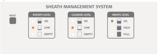
When the waste fluid level is high, the green OK LED changes to a flashing amber LED beside the HIGH label:
