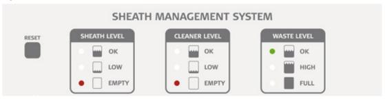
When the waste fluid level changes from high to full, the flashing amber LED changes to a red LED beside the FULL label:
