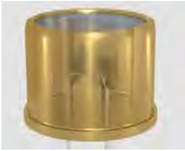
Avalanche Photodiode Detector from the CytoFLEX
