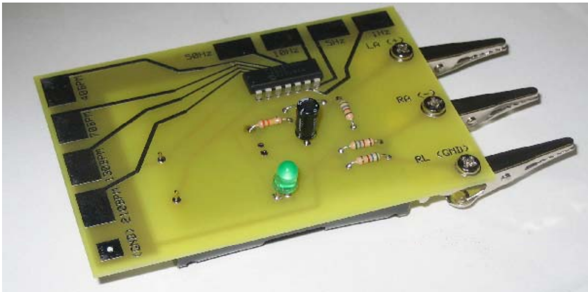
Figure 1a: Front of board with alligator clips for ECG leads on right and switch inputs on the top and left of device
