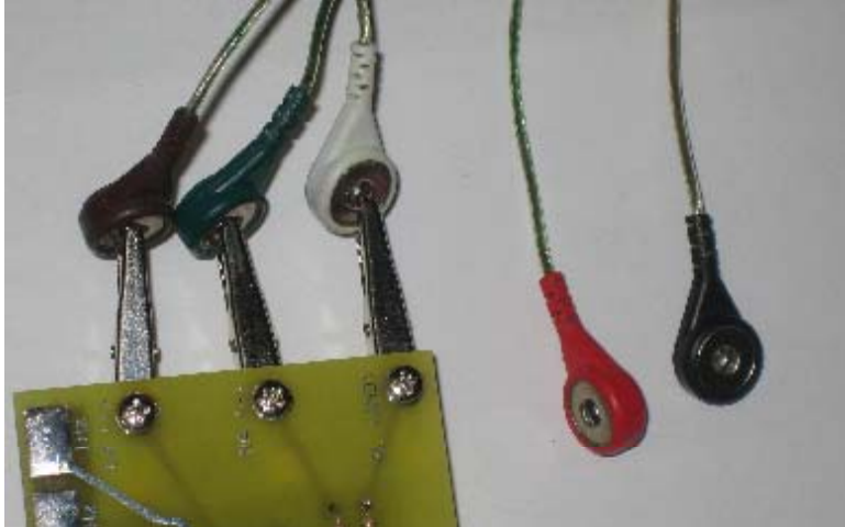
Figure 2b. Attachment of device to a five-lead ECG machine
