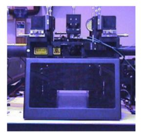
The Aerosol Evacuation System evacuates microdroplets and airborne particulates generated in the sort chamber during the normal jet-in-air operation of the MoFlo cytometer. A simple remote unit controls the system.
