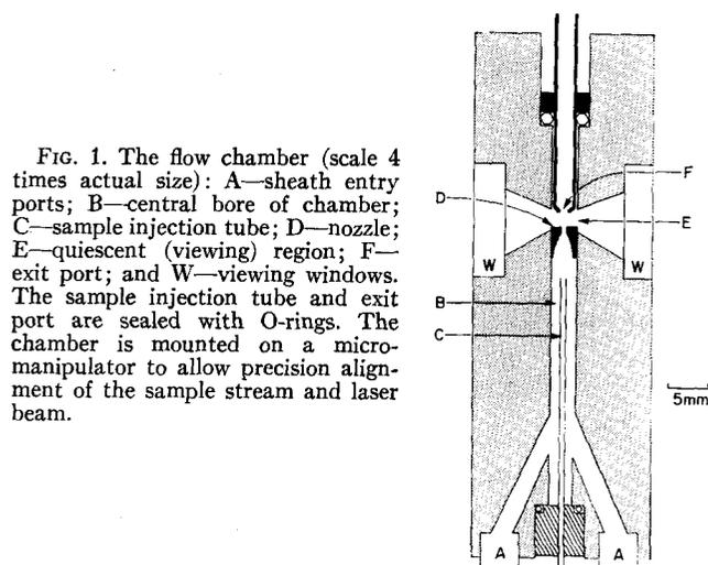
FIG. 1. The flow chamber (scale 4 times actual size): A—sheath entry ports; B—central bore of chamber; C—sample injection tube; D—nozzle; E—quiescent (viewing) region; F—exit port; and W—viewing windows. The sample injection tube and exit port are sealed with O-rings. The chamber is mounted on a micro-manipulator to allow precision alignment of the sample stream and laser beam.
