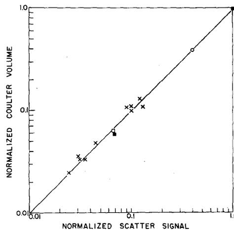
FIG. 2. Comparison of Coulter volume and scatter signal for various samples of plastic microspheres normalized to ragweed pollen: (x)—Dow latex spheres; (O)—3M Corporation carbonized plastic spheres; (■)—Dow latex spheres dyed black; and (□)—the same Dow latex spheres undyed.
