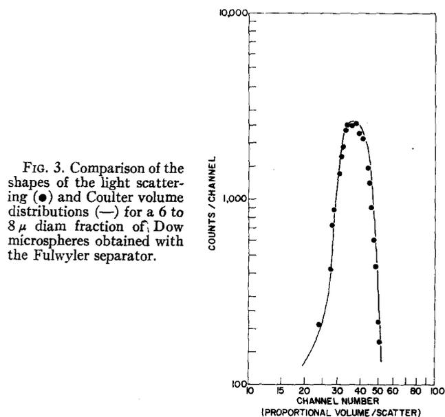
FIG. 3. Comparison of the shapes of the light scattering (●) and Coulter volume distributions (—) for a 6 to 8  $\mu$  diam fraction of Dow microspheres obtained with the Fulwyler separator.
