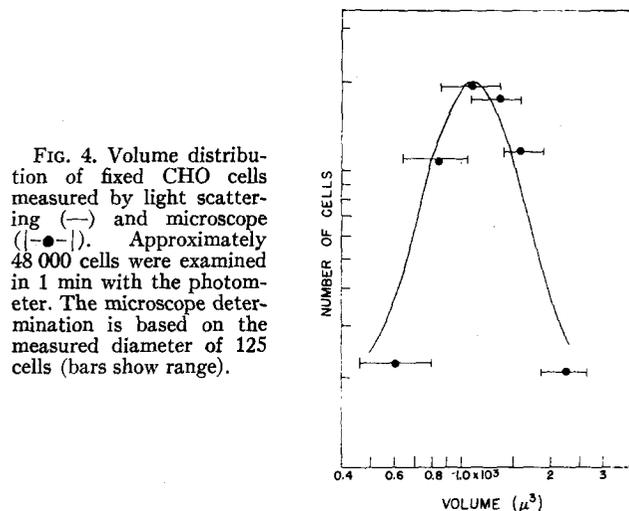
FIG. 4. Volume distribution of fixed CHO cells measured by light scattering (—) and microscope (●—). Approximately 48 000 cells were examined in 1 min with the photometer. The microscope determination is based on the measured diameter of 125 cells (bars show range).
