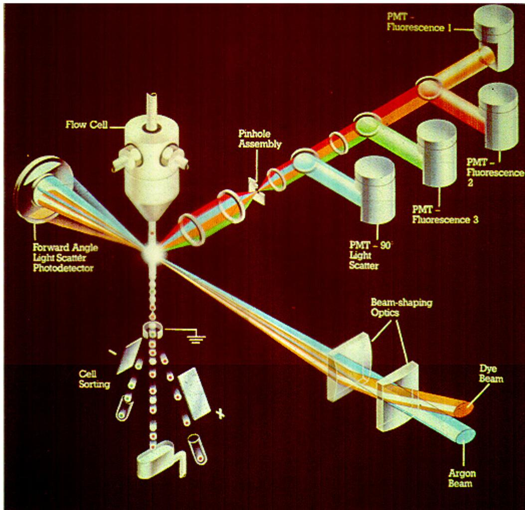
Figure 2: Detection system of a generalised “five parameter” laser based flow cytometer
