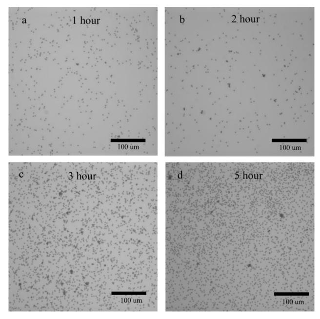
**Figure 3.** Bright field of images of 2.8- $\mu$ m anti-*Listeria* antibody-coated microbeads in PBS buffer (pH 7.2) in contact with a bare C<sub>18</sub> surface for (a) 1 h, (b) 2 h, (c) 3 h, and (d) 5 h. (Scale bar is 100  $\mu$ m.)
