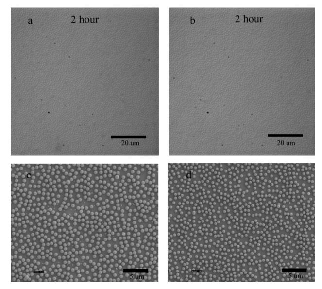
**Figure 5.** Phase contrast images of (a) 0.8-µm polystyrene beads and (b) 0.8-µm dimethylamino beads in PBS buffer (pH 7.2) in contact with C<sub>18</sub> surface pre-adsorbed with BSA for 2 h. (Scale bar is 20 µm.) SEM of (c) polystyrene beads and (d) dimethylamino beads. (Scale bar is 5 µm.)
