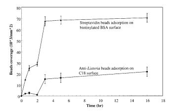
**Figure 4.** Adsorption kinetics of streptavidin microbeads on a  $C_{18}$  surface pre-adsorbed with biotinylated BSA and of anti-*Listeria* antibody-coated microbeads on a bare  $C_{18}$  surface. (Error bar represents one standard deviation in 10<sup>3</sup> beads/mm<sup>2</sup> using data in triplicate.)
