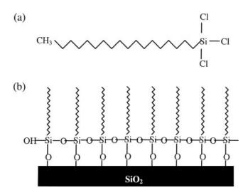
**Figure 1.** (a) Structure of octadecyltrichlorosilane ( $C_{18}$ ). (b) Possible structures of  $C_{18}$  monolayer on the SiO<sub>2</sub> surface. (Drawing is not to scale.)
