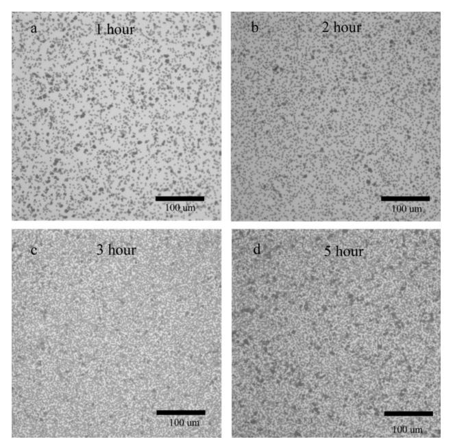
**Figure 2.** Bright field of images of 2.8- $\mu$ m streptavidin-coated microbeads in PBS buffer (pH 7.2) in contact with C<sub>18</sub> surface pre-adsorbed with biotinylated BSA for (**a**) 1 h, (**b**) 2 h, (**c**) 3 h, and (**d**) 5 h. (Scale bar is 100  $\mu$ m.)
