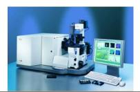
CompuCyte's iCys® Research Imaging Cytometer utilizes proprietary laser scanning technology to enable quantitative measurements of cellular biochemical constituents and simultaneous evaluation of cell morphologies. The technology allows automated analysis of solid-phase samples, including adherent cultured cells, tissue sections, tissue microarrays, tissue imprints, and cytology specimens stained with fluorescent and chromatic dyes. For more information please visit www.compucyte.com.
