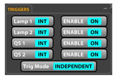
The Trig Mode is used when one lamp is fired by an external trigger and the second lamp is set to internal.
