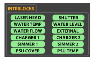
If the laser won't start, it may be due to an interlock fault. Check the interlock indicators to ensure they are green.
