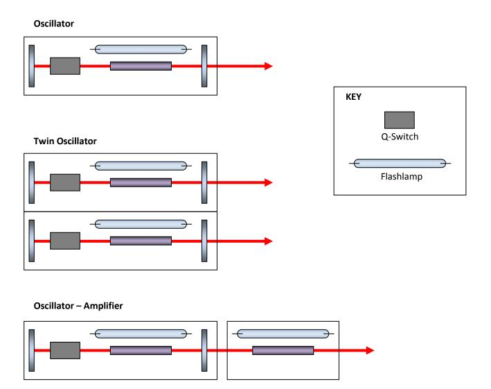
Each Oscillator has a flashlamp which is triggered to fire a pulse of energy into the laser rod. This pulse is typically a few hundred microseconds in length. When enabled, the q-switch can be triggered after the flashlamp to let the laser pulse out of the laser cavity. The timing of these triggers is discussed later.
