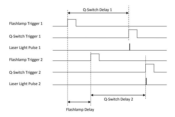
The flashlamp delay may be positive or negative enabling the lasers to fire in any order. A positive delay will cause Laser 1 to fire before Laser 2. A negative delay results in Laser 2 firing first.
