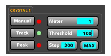
Track mode is useful on system where the optimum angle of the harmonic crystal changes over time due to absorption or other effects.
