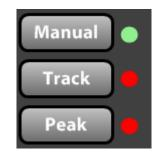
There are three possible modes used to remotely tune a harmonic crystal. These modes are selected using the MANUAL, TRACK and PEAK buttons.
